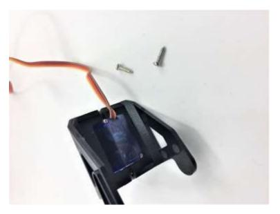
Use two self-tapping screws (in the FPV package) to tighten
