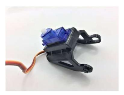
Assemble the FPV holder and servo
