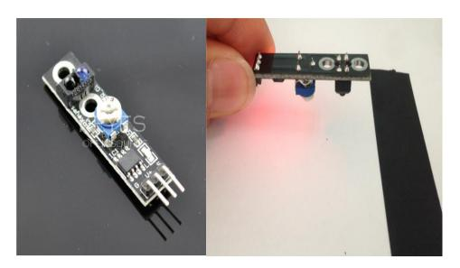
The adjustable resistor on Module is used to adjust the sensitivity, adjust to the appropriate location, here to teach you how to adjust. Find a piece of white paper, with black tape. Connect the tracking module to the power supply only to VCC and GND. Put the module in the paper about 1CM, swing it between white and black, watching if the red light on the module has a change, if not change, adjust the variable resistor. When the module doesn't encounter the black line, red light is on.
