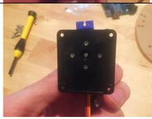
9. Take the other two pieces of the servo holder and snap them onto the servo (there are grooves in the side pieces that match the plastic tab on the servo).
