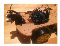
13. Use four short screws to attach the upper part of the chassis to the copper shafts. Set the six-AA battery holder on top of the chassis (screw it down if you can), attach the 9V cell holder to the Arduino.
