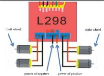
4. Fixed and wiring up the power supply (battery box) on the board wiring up the.
