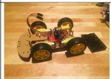
12. Now it's time to start putting this thing together. Grab the upper part of the chassis and set it on top of the copper shafts connected to the lower part, and pull the wires attached to the H-bridge through the hole in the center of the chassis. Connect the six wires to I/O ports as follows:
