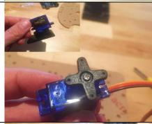
8. Then flip the servo upside down into the black plastic ring of the holder. Make sure that the wires coming out of the servo are facing in the same direction as the longer part of the holder (again, see the image below), and use four tiny screws to secure the crossbar (there are four holes in the holder that align with the holes on the crossbar). Here's what it looks like after it's attached.
