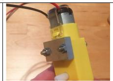
2. Now each motor can be attached to the chassis by using two short bolts in the bottom of each metal bracket. Here's a view of the bottom of the chassis so you can see where the bolts need to be.
