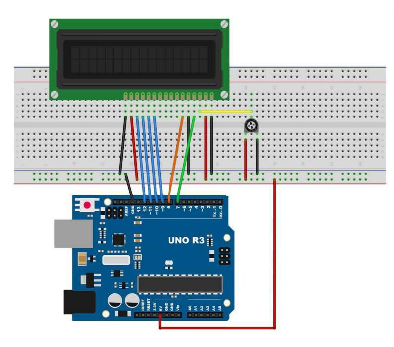
The LCD display needs six Arduino pins, all set to be digital outputs. It also needs 5V and GND connections.
