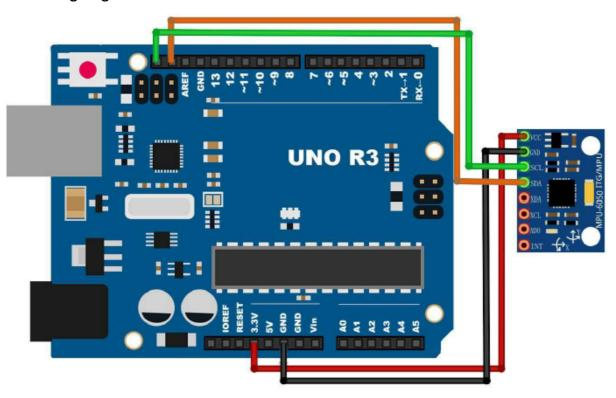
Next, we need to set up the I2C lines. For this connect the pin labelled as SDA on the GY-521 to the Arduino's analog pin 4 (SDA). And the pin labelled as SCL on the GY-521 to the Arduino's analog pin 5 (SCL). And that's it, you have finished wiring up the Arduino GY-521.
