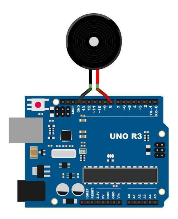
Wiring the buzzer connected to the UNO R3 board, the red (positive) to the pin8, black wire (negative) to the GND.
