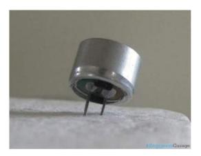
These microphones are widely used in electronic circuits to detect minor sounds or air vibrations which in turn are converted to electrical signals for further use. The two legs as shown in the image above are used to make electrical connection with the circuit.
