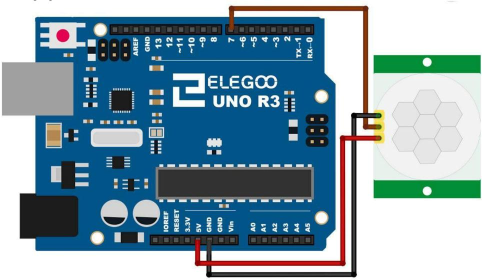
Connecting PIR sensors to a microcontroller is really simple. The PIR acts as a digital output so all you need to do is listen for the pin to flip high (detected) or low (not detected).
