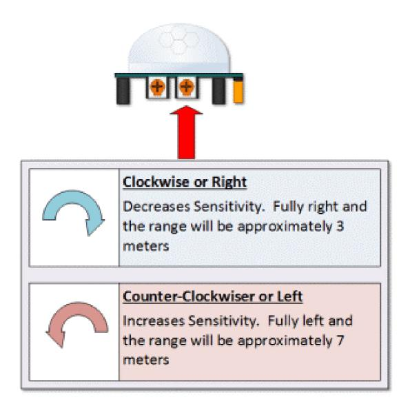
HC SR501 Sensitivity Adjust Time Delay Adjustment
