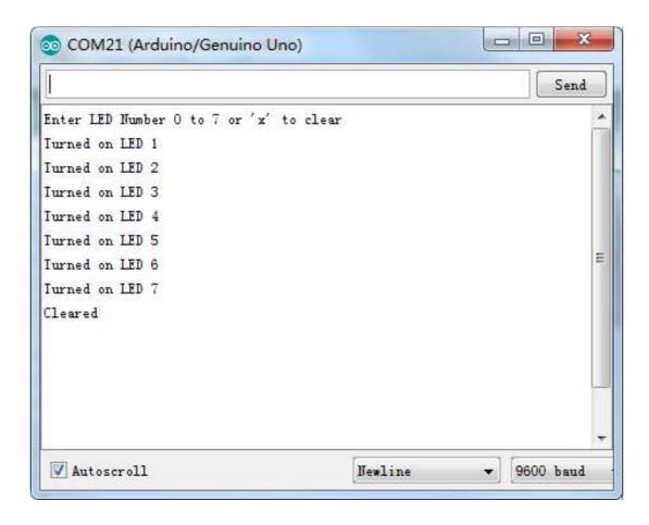
Type x again and press 'Send' to turn off all LEDs.
