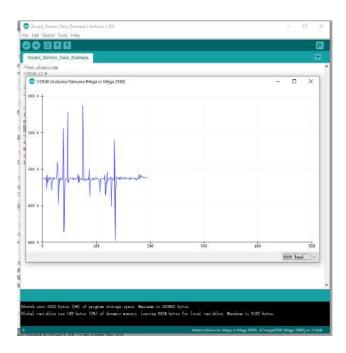
When you speak into the microphone or inflate, you can observe that our waveforms have changed The following is the procedure required to use this experiment and notes to explain:
