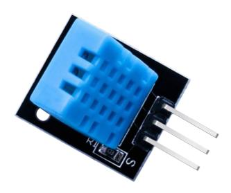
DHT11 digital temperature and humidity sensor is a composite Sensor which contains a calibrated digital signal output of the temperature and humidity. The dedicated digital modules collection technology and the temperature and humidity sensing technology are applied to ensure that the product has high reliability and
