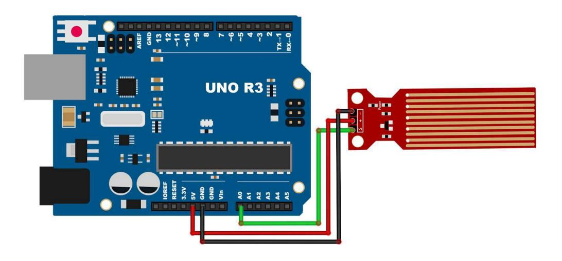
Wiring tips: Power supply (+) is connected to 5V of UNO R3 board, ground electrode (-) is connected to GND. Signal output (S) is connected to the ports (A0-A5) which have function of inputting analog signal in UNO R3 board, random one is OK, but it should define the same demo code as the routine.
