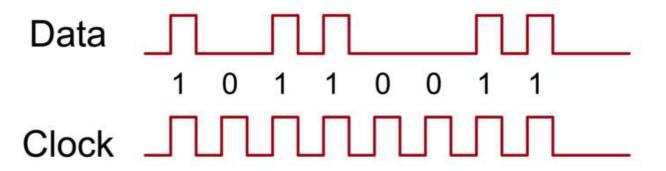
The clock pin needs to receive eight pulses. At each pulse, if the data pin is high, then a 1 gets pushed into the shift register; otherwise, a 0. When all eight pulses have been received, enabling the 'Latch' pin copies those eight values to the latch register. This is necessary; otherwise, the wrong LEDs would flicker as the data is being loaded into the shift register.
