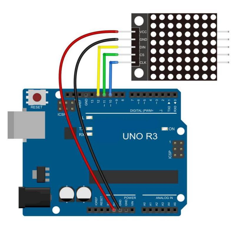
VCC and Ground are connected to the Arduino.
