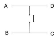
Actually, there are only really two electrical connections. Inside the switch package, pins B and C are connected together, as are A and D.
