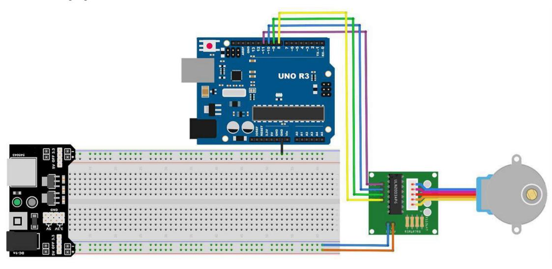
We are using 4 pins to control the Stepper.
