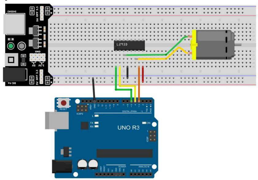
The code below does not use a separate power supply (ie a battery), it uses instead the 5v power from the Arduino. Note that this would be risky without the L293D controlling it.
