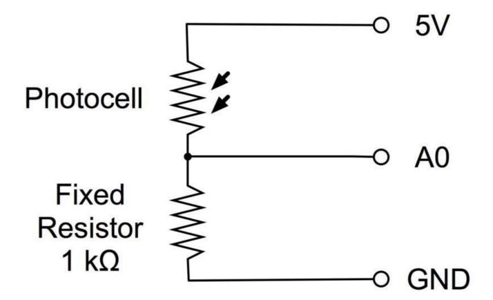
The resistor and photocell together behave like a pot. When the light is very bright, then the resistance of the photocell is very low compared with the fixed value resistor, and so it is as if the pot were turned to maximum.
