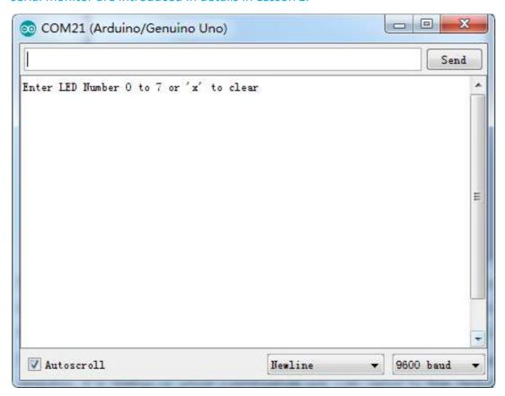
This window is called the Serial Monitor and it is part of the Arduino IDE software. Its job is to allow you to both send messages from your computer to an UNO board (over USB) and also to receive messages from the UNO.
