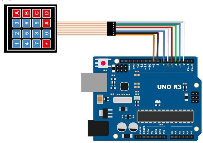
When connecting the pins to the UNO R3 board, we connect them to the digital output pins, D9-D2. We connect the first pin of the keypad to D9, the second pin to D8, the third pin to D7, the fourth pin to D6, the fifth pin to D5, the sixth pin to D4, the seventh pin to D3, and the eighth pin to D2.
