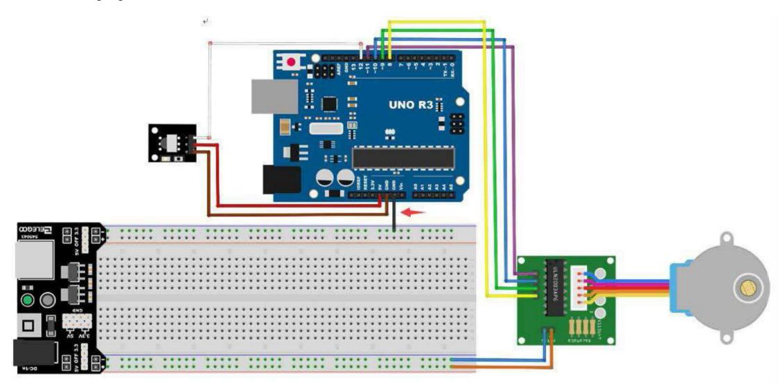
We are using 4 pins to control the Stepper and 1 pin for the IR sensor.
