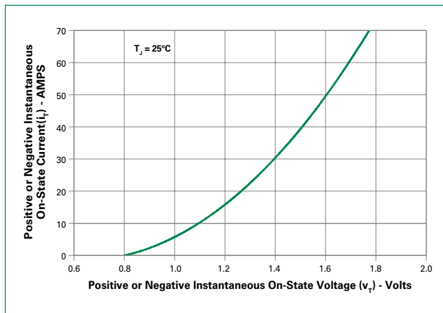
Figure 9: On-State Current vs. On-State Voltage (Typical)
